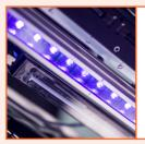
UV-LED Pinning and UV Final Cure UV-LED pinning system custom designed and developed by Inca. Uses proven UV-LED technology with life expectancy exceeding 20,000 hours, reducing heat exposure to sensitive substrates, improving the drop registration and the overall print quality. Individually switchable UV-LED pinning for zero UV masking. Final UV cure through a tunnel provides excellent adhesion and durability.
